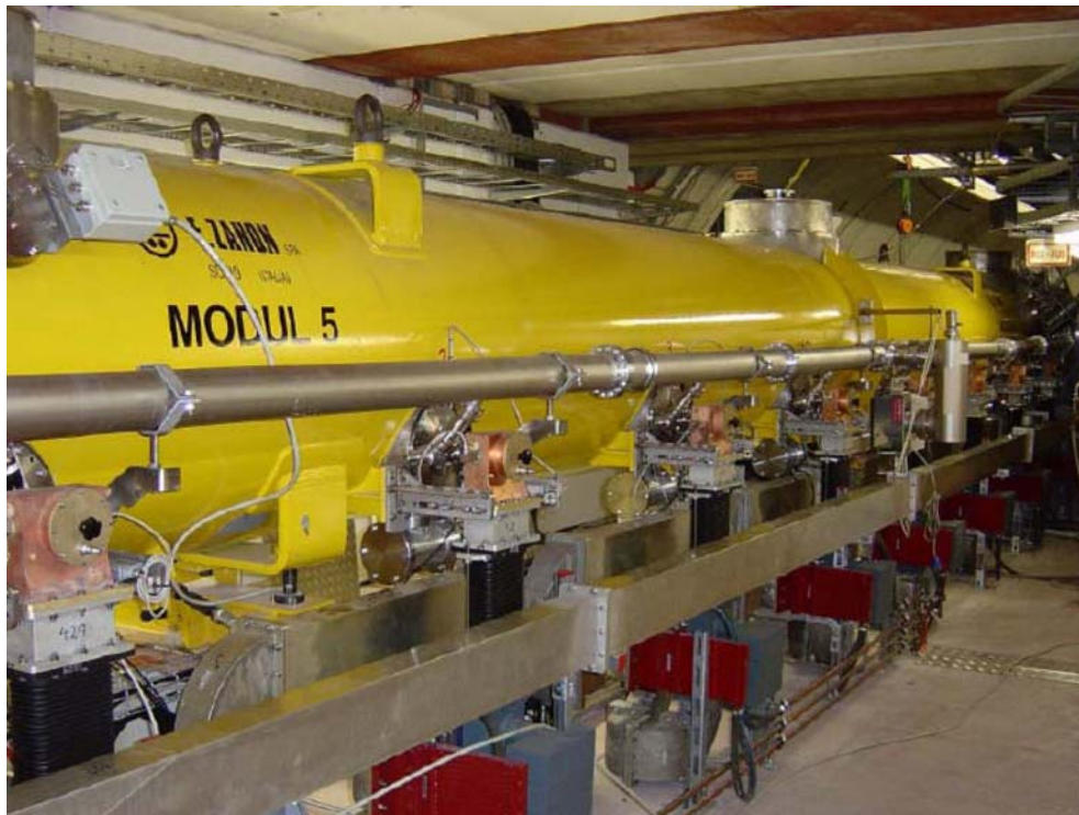
Fig. 1.10: A TESLA cryo-module as will be the basis of the BESSY FEL linac.
