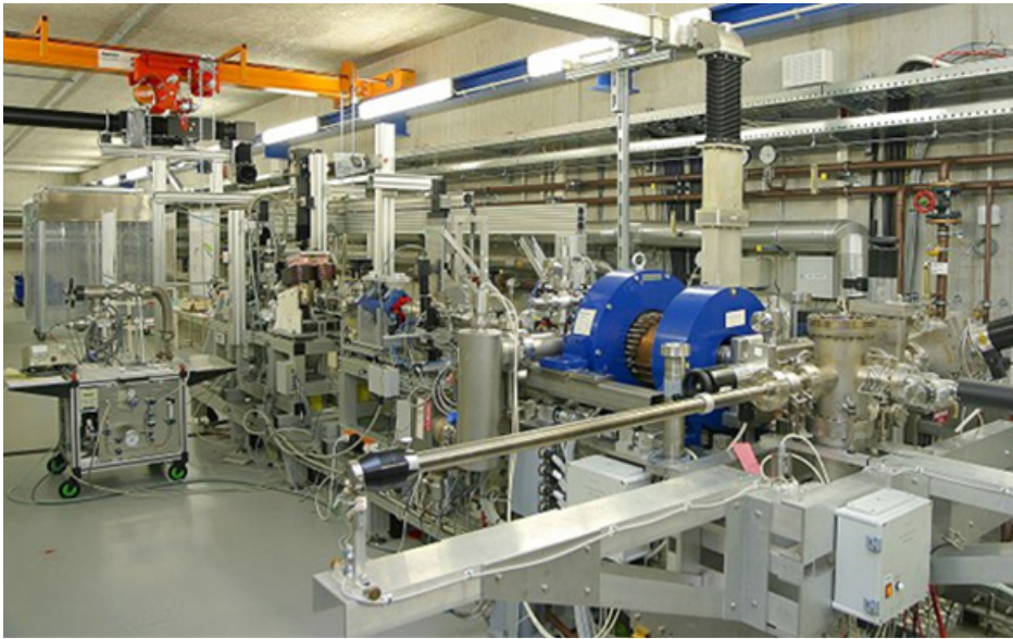
Fig. 5.4: The PITZ photoinjector as in late 2003. The two solenoids (main solenoid and bucking coil in blue are clearly visible with the RF cavity herein). In the foreground is the cathode exchange system.
