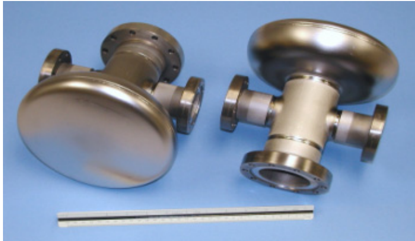
Fig.5.32: The all-niobium BNL s.c. gun cavity design (photograph taken from [23]).
