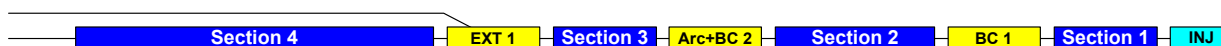
Fig. 15.10: Layout of the BESSY FEL (INJ: injector; BC: bunch compressor; EXT: extraction point)
