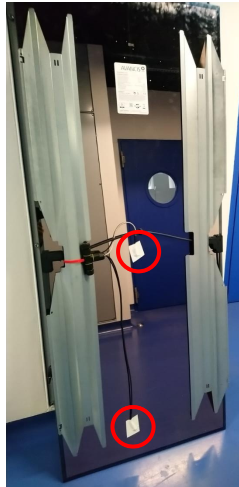
Figure 5: Temperature sensors on the solar module rear side (circled in red)
