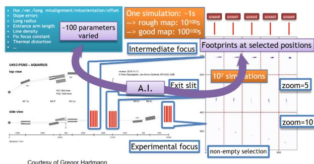
Figure 7: Surrogate models of the beamlines generated with machine learning methods (AI) are more efficient in process tuning than e.g. ray tracing predictions.
