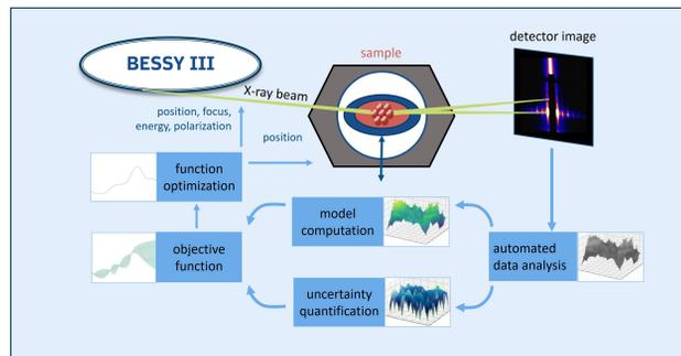
Figure 8: A schematic of autonomous experimentation balancing exploration, i.e. learning the landscape of the parameter space, approaching the objective function, and exploitation, i.e. attempting to rapidly achieve relevant results, trying functions as optimized. Sample model development and uncertainty removal are best guided by simulations and checked against FAIR data bases.
