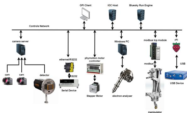
Figure 4: Complex device variety at instruments.
